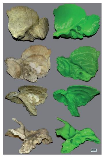
Fig. 1. Original temporal bone (left) and printed polymer replica (right) seen in various orientations.
