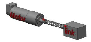
Figure 3: Single-link manipulator with a flexible joint
