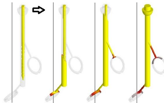
Fig. 4. Visualization of 4 stages of the process simulation, indicating the unexpectedly rapid course of solidification at the end of filling and the formation of misruns in both elements (the metal has solidified before filling the mould cavity)
