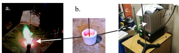
Fig. 6. Elements of workplaces for thermal analysis: a - propane-butane burners, b - 15 cm<sup>3</sup> ceramic crucible and K-type thermocouple, c - laboratory furnace with capacity of 1200W,  $T_{max} = 1150^{\circ}\text{C}$
