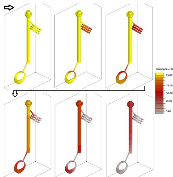
Fig. 9. Selected stages of simulation of solidification of ring and signet out of Au-Ag-Cu alloy (+Zn), discretization grid  $\Delta x = 0.5$  mm
