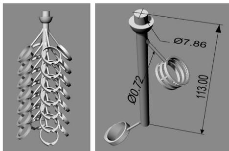
Fig. 3. Complete sets ("trees") of cast elements, (left: typical layout for serial production, right: simplified layout containing 2 elements, see Figure 1)
