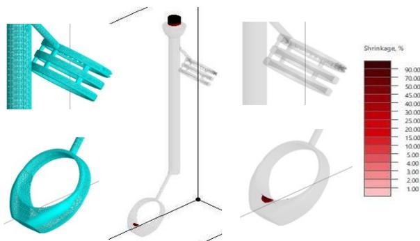
Fig. 10. Forecast of shrinkage defects in the raw cast of the ring and the signet and fragments of the 3D mesh model ( $\Delta x = 0.5$  mm)
