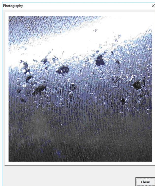
Fig. 5. Example of visualisation of the "shrinkage porosity" defect in the Open Atlas of Defects
