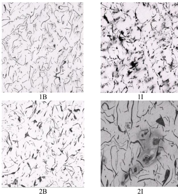
Fig. 1. Microstructure of the thickest portion of the samples (Mag.100x, unetched)
