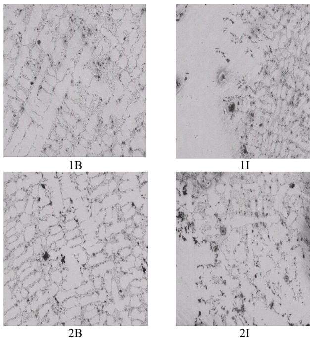
Fig. 2 . Microstructure of thinnest portion of the samples (Mag.100x, unetched)
