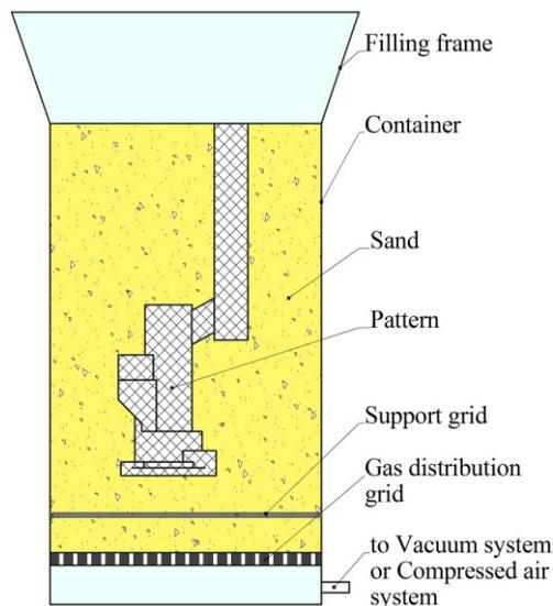
Fig. 2. Container with pattern block
