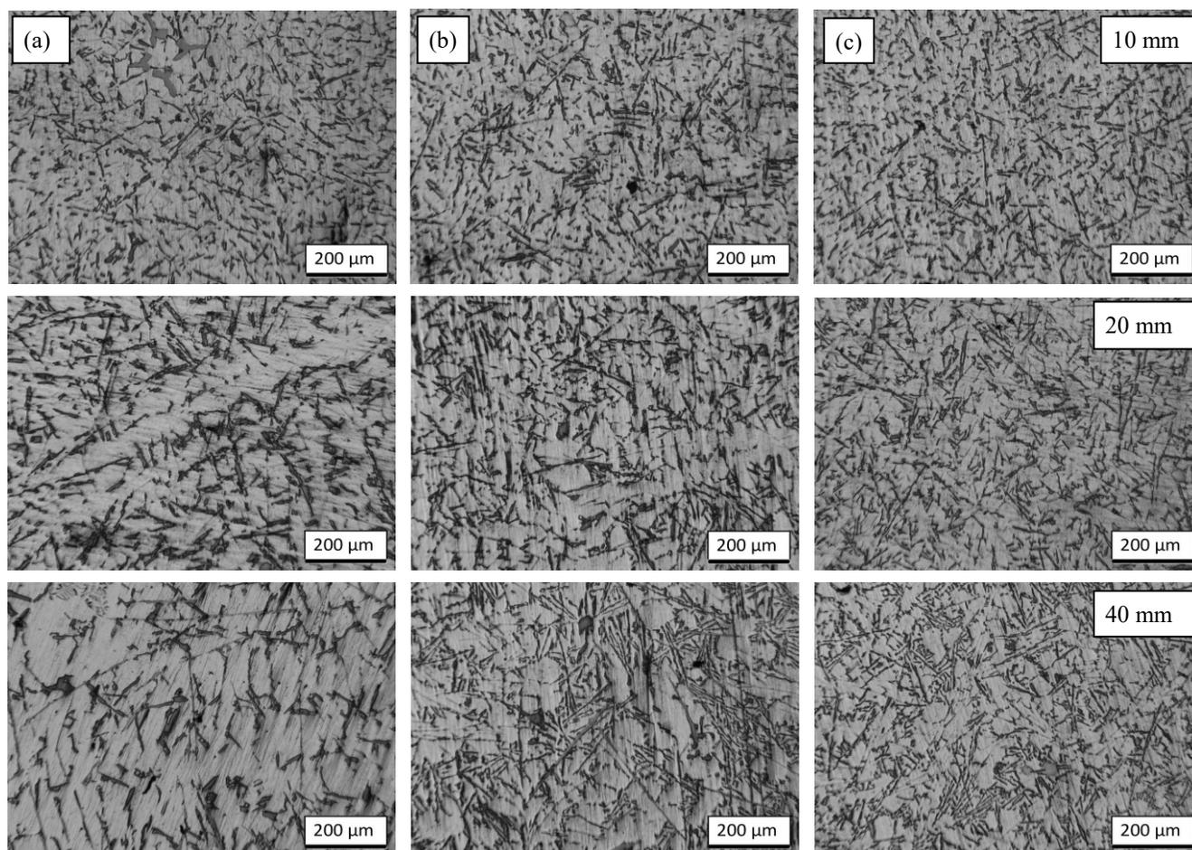
Fig. 3. Microstructure of different wall thickness of castings obtained by conventional LFC technology (a), technology with sand fluidization mode B (b) and mode C (c)
