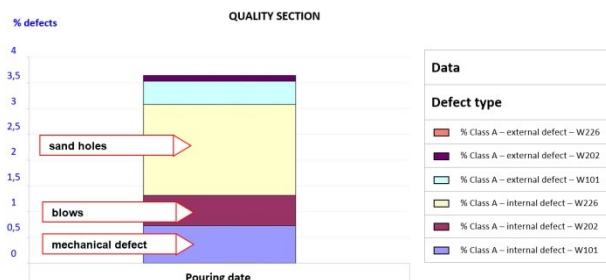
Fig. 3. Chart generated by the A&DM system on the percentage share of the 3 key assortment defects for 1 week
