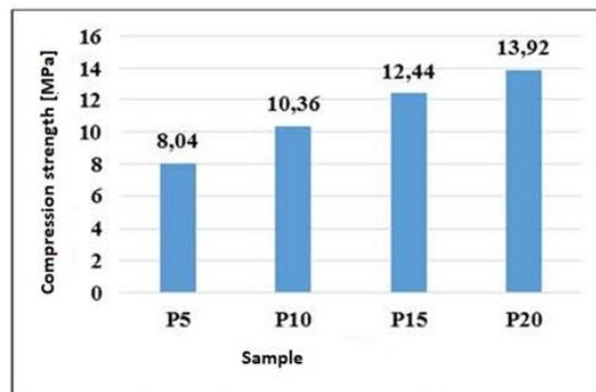
Fig. 5. Average values of the compression strength of compounds P5 ÷ P20
