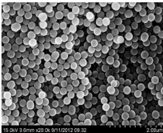
Fig. 3. Aluminosilicate microspheres [19]
