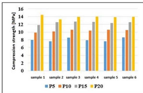
Fig. 4. Compression strength of samples 1÷6 of compounds P5÷P20
