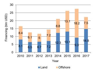
Fig. 3. Financing of new wind investments on land and at sea in 2010–2017 in billions of USD; source: own elaboration based on WindEurope [2018b]
