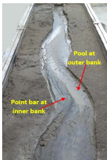
Fig. 3. Formation of pool-point bar unit for experiment run A-4 at t = 480 min; source: own elaboration
