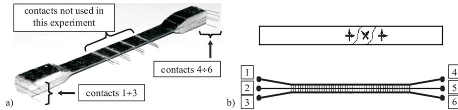
Fig. 3. View of specimen for tension examination: a) general view and position of contacts, b) enumeration of contacts
