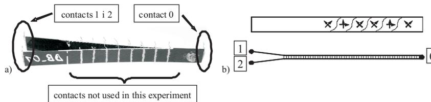
Fig. 5. View of specimen for delamination examination: a) general view and position of contacts, b) enumeration of contacts
