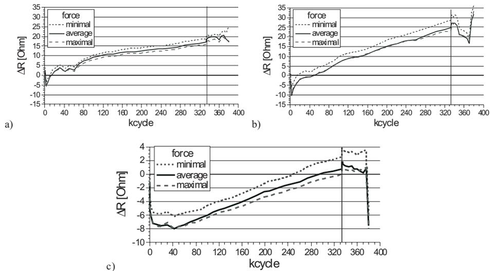
Fig. 11. Change of resistance between measurement points in cyclic load test for: a) point p-1; b) point p+1; c) point p0 (description in this Section)
