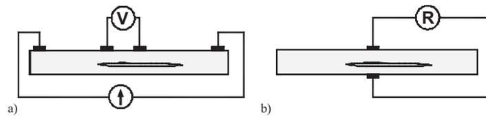
Fig. 2. Methods of examining electrical properties of composite: a) measurement of potential change, b) measurement of resistance change
