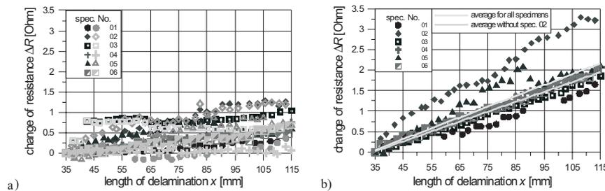
Fig. 6. Changes of resistance between measurement points in delamination test: a) points 0 – 1 and 0 – 2, b) points 1 – 2
