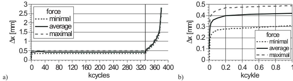
Fig. 10. Displacement of bolt in cyclic load test (description in this Section)
