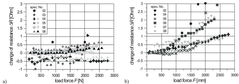
Fig. 4. Changes of resistance between measurement points in tension test: a) between points 1-4 and 3-6, b) between points 2-5
