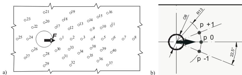
Fig. 8. Allocation of measurement points in destruction test of bolt joint: a) quasi-static test, b) fatigue test
