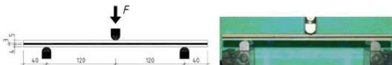
Fig. 2. Test bench scheme and the sample geometry in bending
