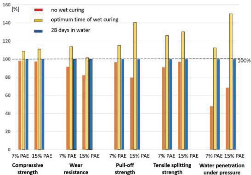
Figure 11. The influence of curing conditions on the properties of 28-days old PCC modified with PAE (red bars - no curing, yellow bars - optimum time of wet curing, blue bars - 28 days in water)
