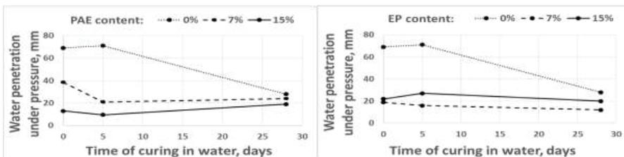
Figure 8. Wet curing time vs water penetration under pressure of PCC with PAE (a) and EP (b). Test performed for 28-days old concrete
