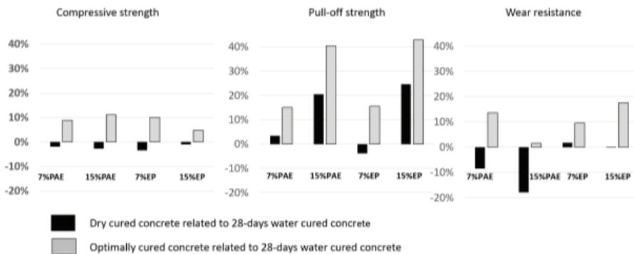
Figure 10. Results of testing at the age of 28 days: compressive strength, wear resistance and surface tensile strength
