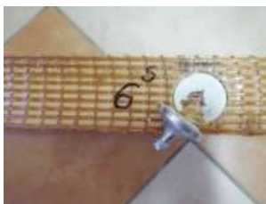
Fig. 5. Adhesive failure between the adhesive layer and the disc.
