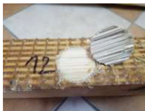
Fig. 6. Cohesive failure in the substrate.
