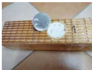
Fig. 4. Adhesive failure between the adhesive layer and the disc
