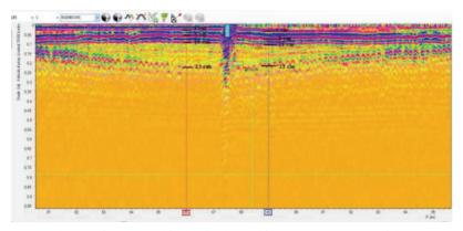
Fig. 8. Radagram at Bridge Deck Joint 1 with 2GHz antenna at 88 m joint.
