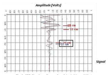
Fig. 9. GPR Signal at a distance from Joint 1 (86m and 89m).
