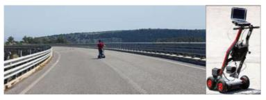
Fig. 2. Ground coupled GPR survey during the bridge monitoring.
