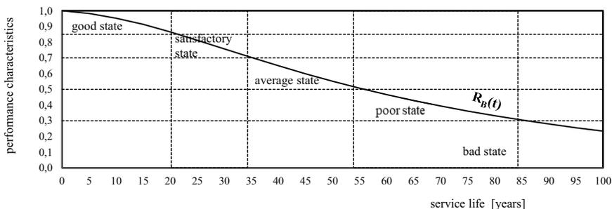
Fig. 1. Changes in performance characteristics of a building described by the PRRD model.
