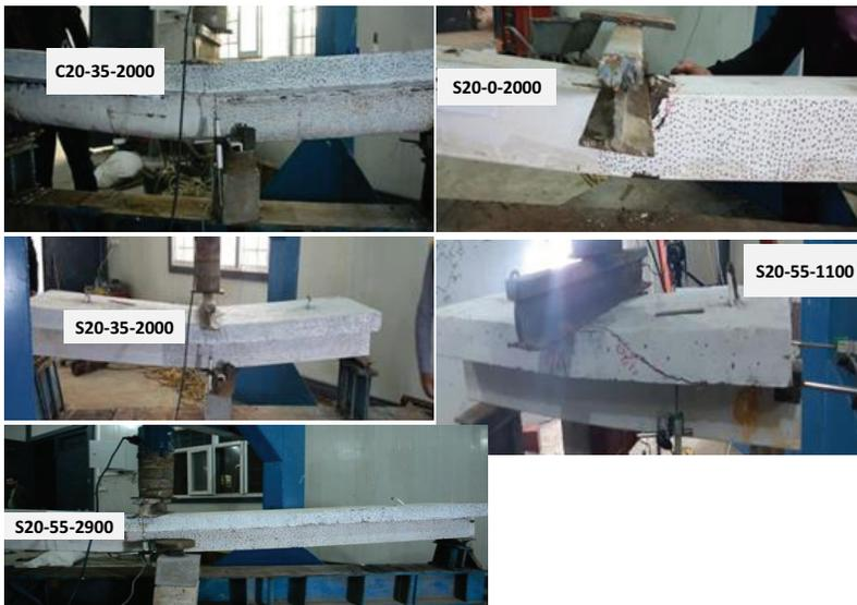
Fig. 5. Specimens during and after the test.
