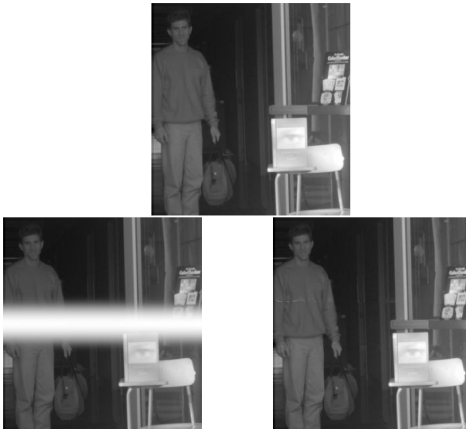
Fig. 14. The effect of folded multiple capture for achieving high dynamic range. The three images are as follows: Top: image of HDR scene. Bottom left: simulated image with moving laser. Bottom right: simulated image using FMC with disturbance tolerance (After Ref. 42).
