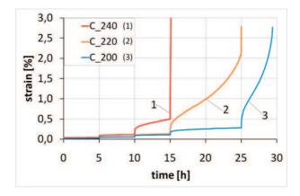
Fig. 4. Comparison of the creep curves for the low porosity AlSi8Cu3 tested at three selected temperatures: 200°C (C 200), 220°C (C 220), 240°C (C 240)
