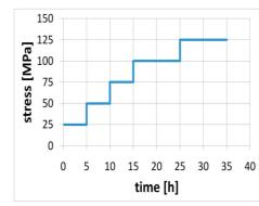
Fig. 2. Programme of creep tests
