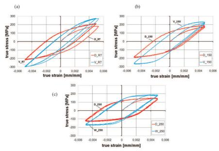
Fig. 8. Hysteresis loops for first two cycles of the block with amplitude ±0,005 (3) for:
