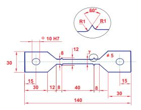
Fig. 1. Specimen used for creep tests
