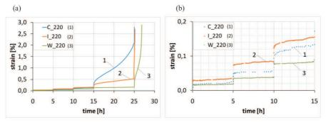
Fig. 3. Comparison of the creep curves for: low porosity AlSi8Cu3 (C\_220), high porosity AlSi8Cu3 (I\_220) and low porosity AlSi7MgCu0.5 (W\_220) tested at 220°C; (a) – full creep curves; (b) – magnified view of curves at period from 0 to 15 [h]
