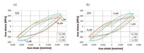
Fig. 7. Hysteresis loops for first two cycles of the block with amplitude  $\pm 0,005$  (3) for: low porosity AlSi7MgCu0.5 (V\_150), low porosity AlSi8Cu3 (D\_150) and high porosity AlSi8Cu3 (I\_150), tested at 150°C with the following sequences of blocks: (a) 123 and (b) 231
