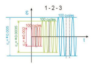
Fig. 6. Programme of LCF tests
