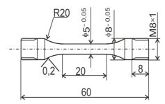
Fig. 5. Specimen used for LCF tests
