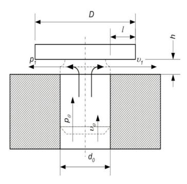
Fig. 1. Pressure emulsifying valve D – valve diameter,  $d_0$  – valve seat orifice diameter,  $v_0$  – fluid flow velocity at the entrance to the valve seat orifice,  $p_0$  – pressure at the entrance to the valve seat orifice,  $v_1$  – fluid flow velocity at the valve seat orifice outlet,  $p_1$  – pressure at the valve seat orifice outlet, h – gap height, l – gap length
