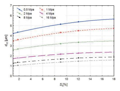
Fig. 5. Relationship between characteristic dimension  $d_{cz}$  of dispersed-phase particles and dispersed-phase content  $S_v$  in emulsion. Emulsifying temperature  $t = 20^{\circ}$ C, and emulsifying pressures p = 0.5, 1, 2, 4, 8 and 16 MPa
