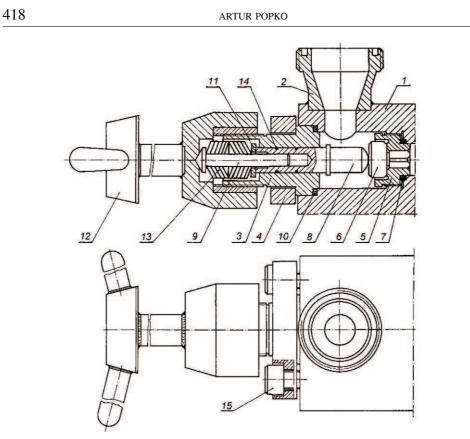
Fig. 3. Construction of emulsifying head of pressure emulsifier CHO- 03 M [11] 1 – body of the block, 2 – outlet connector pipe, 3 – running unit, 4 – fixing plate, 5 – valve seat, 6 – valve, 7 – seal, 8 – piston, 9 – tappet, 10 – seal of the unit, 11 – pad of the spring, 12 – knob, 13 – spring, 14 – sealing ring, 15 – fixing screw
