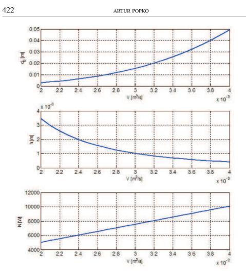
Fig. 8. Characteristics of establishing construction-exploitation parameters of emulsifying valve and determining the power demand of the emulsifier necessary for scattering of the dispersed-phase particles
