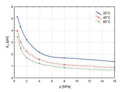
Fig. 4. Dependence of characteristic dimension  $d_{cz}$  of dispersed-phase particles on emulsifying pressure *p*. Data are shown for  $S_v = 9\%$  of dispersed phase. Temperatures of emulsifying are: t = 20, 40 and  $60^{\circ}$ C
