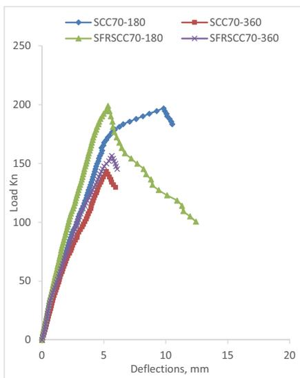
Figure 9(a): Load vs. deflections for SCC 70; 8mm
