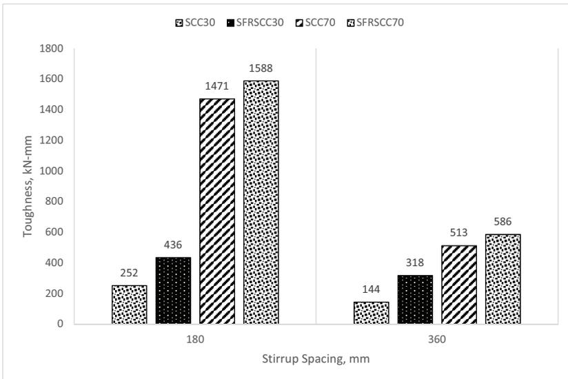
Figure 7: Toughness vs. stirrup spacing for 8mm  $\varnothing$  stirrup
