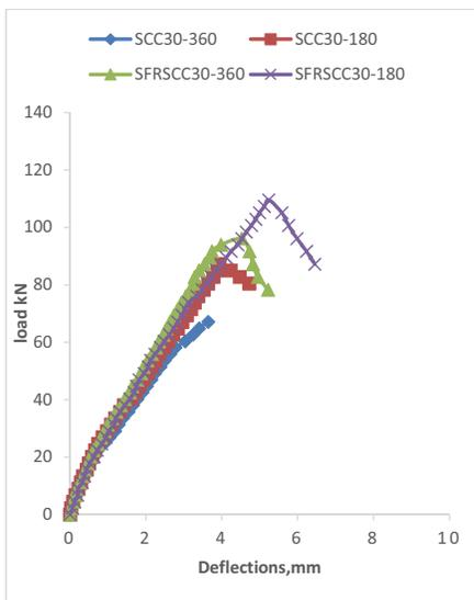
Figure 8(a): Load vs. deflections for SCC 30; 8mm  $\sigma$  stirrup
