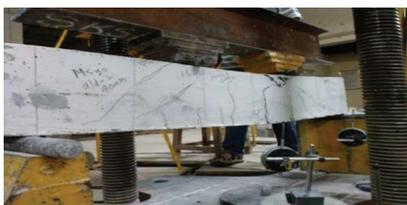
Figure 11 Failure pattern of SFSCC30
