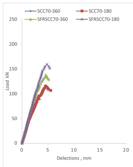
Figure 9(b): Load vs. deflections for SCC 70; 6mm
