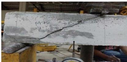
Figure 12: Failure pattern of SCC70
