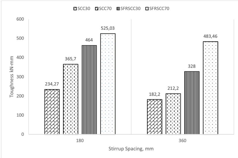
Figure 6: Toughness vs. stirrup spacing for 6mm  $\varnothing$  stirrup
