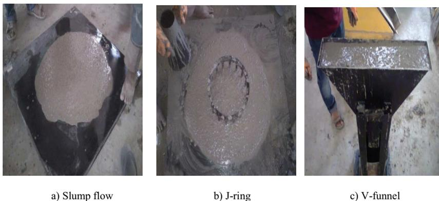
Figure 3: Some tests on the workability of SCC
