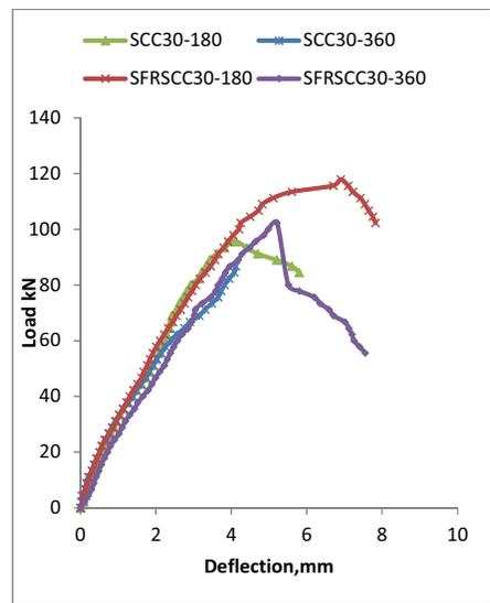
Figure 8(b): Load vs. deflections for SCC 30; 6mm  $\sigma$  stirrup
