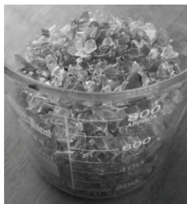
Fig. 1. Left: Volumetric composition of tested composites: CM – cement mortar, PCC – polymer-cement composite (where 0%, 10%, 20% and 25% means the content of PET in the total aggregate volume), right: the finest (fraction 0-4 mm) PET blend
