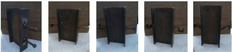
Fig 2. Shear connectors welded to the universal steel beam: (a) Stud, (b) Channel-section, (c) I-section, (d) S-section, and (e) Z-section
