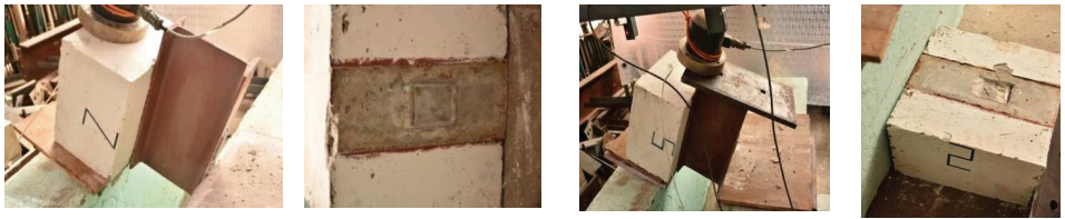
Fig.7. Typical failure of push-out specimens
