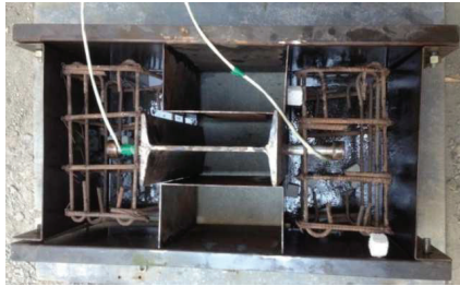
Fig 3. View of concrete casting mould with reinforcements
