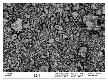
Fig. 1 Irregular ash grains from TTMSS, 200x magnification, BSD technique
