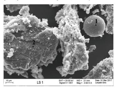
Fig. 2 Ash grains from TTMSS, 2500x magnification, SE technique
