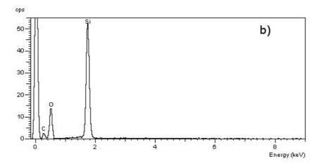
Fig. 3 EDS analysis of areas 1 (a) and 2 (b) - fig. 2
