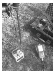
Fig. 4. Panda 2 test rig prepared for testing
