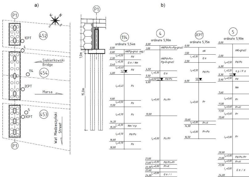
Fig. 3. Comparison of the ground profiles near to the abutment P1; a) location of the boreholes (114 of 1998, 4, 5 of 2016) and of the cone penetration tests (1CPT, 2CPT, 3CPT of 2016); b) borehole profiles
