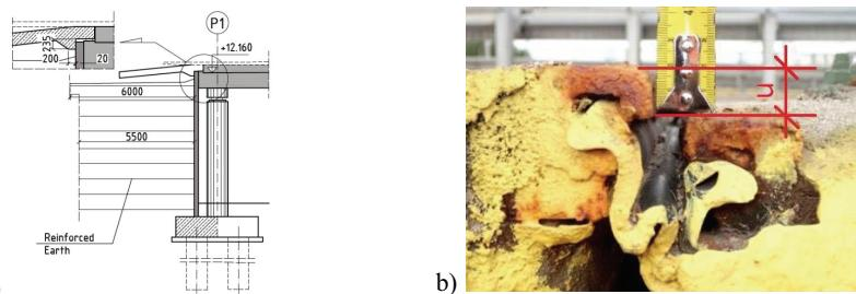
Fig. 4. The abutment P1 [1]; a) a drawing of connection with the approach slab [mm].
