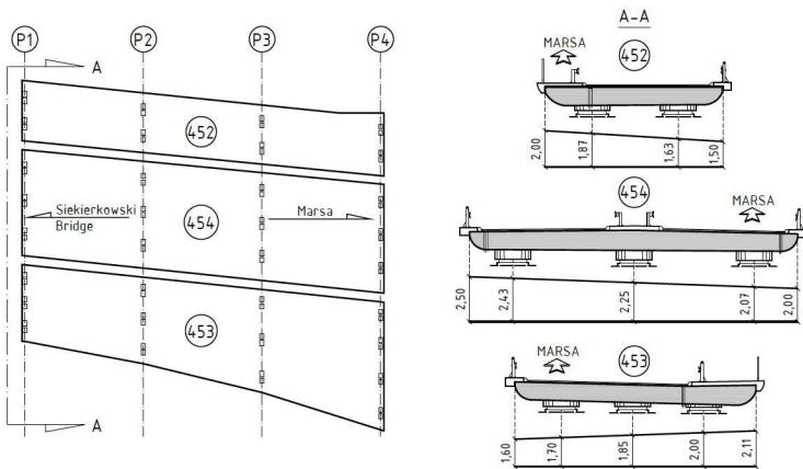
Fig. 5. Superstructures of flyovers [1], [11]; a) plan view of flyovers; b) cross-sections A-A – the measured values of the offset  $u$  [cm]
