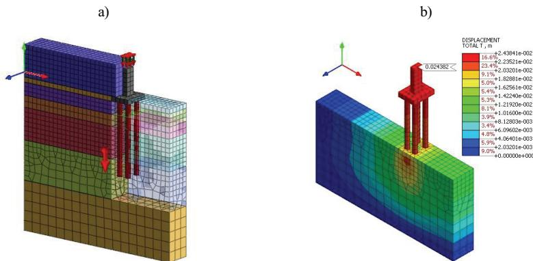
Fig. 7. Calculation model for a group of piles [11]: a) visualization of the model, b) visualization of the exemplary results – total settlement caused by permanent loads and negative friction (red colour denotes maximum values, blue colour denotes minimum values)
