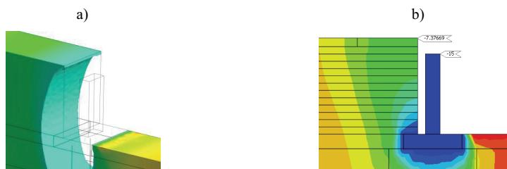
Fig. 9. Examples of the results of the vertical displacement caused by negative friction having the form of forced displacement (settlement of the abutment); a) fragment of 3D model with "cut-out" areas in which the displacement was smaller than occurring at the edge next to the embankment's expansion joint – variant-2; b) displacement of the edge of abutment in case of prescribed displacement of pier, plane strain deformation model (2D)
