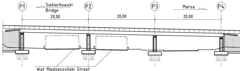
Fig. 2. Side-view drawing of Trasa Siekierkowska route's flyovers stretching over Wał Miedzeszyński Street [1]
