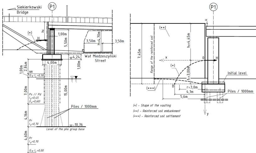
Fig. 10. Analyzed scheme of the abutment P1; a) the geological cross-section; b) outline of the vaulting
