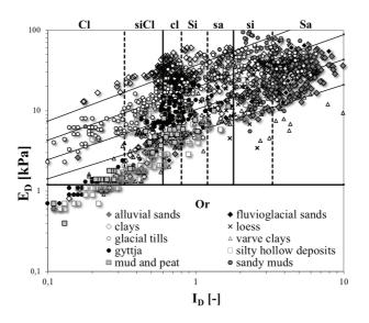
Fig. 2. All results for different test sites for analysed soils plotted on Marchetii's classification nomogram.
