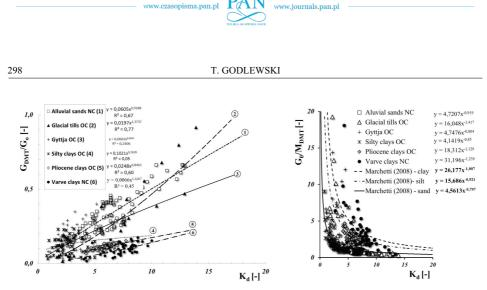
Fig. 4. Graph of the  $G_{DMT}/G_0$  (left) and  $G_0/M_{DMT}$  indicator (right) vs  $K_D$  for chosen types of soils [18] with modifications.
