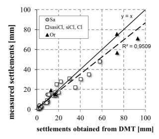
Fig. 3. DMT calibration curve obtained for Polish ground conditions [upgrade from 15]
