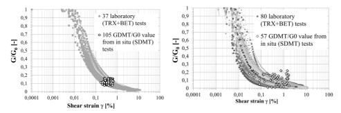
Fig. 5. Shape of the normalized  $G/G_0$ - $\gamma$  degradation curve's range and values of  $G_{DMT}/G_0$ - $\gamma_{DMT}$  based on the SDMT for OC clays (on left) and OC glacial tills (on right).
