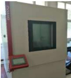
(a) Quick concrete freeze-thaw tester
