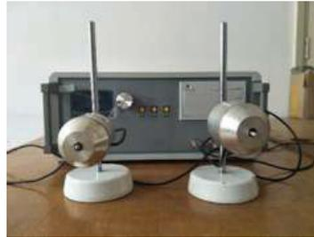
(b) DT-20W dynamic modulus of elasticity of tester
