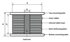
Figure 7. LRB isolator system (after [13]).
