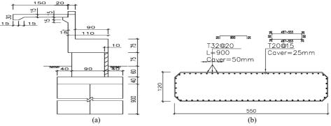
Figure 4. Details of the Hesarak Bridge (uint in cm): a) Abutment, and b) Pier section [16].
