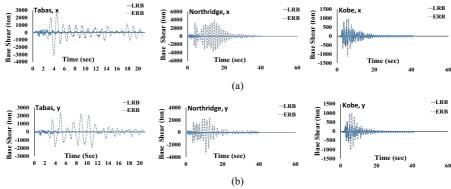
Figure 10. Base shear time history of the bridge due to the three representative earthquake motions: a) Longitudinal direction, and b) Transverse direction.
