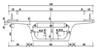
Figure 3. Cross-section through the deck of Hesarak Bridge (uint in cm) [16].
