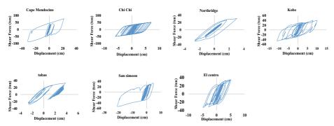
Figure 15. Hysteresis loop for the LRB isolator subjected to the given earthquake motions.
