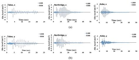
Figure 13. The deck acceleration time history of the bridge due to the three representative earthquake motions: a)
