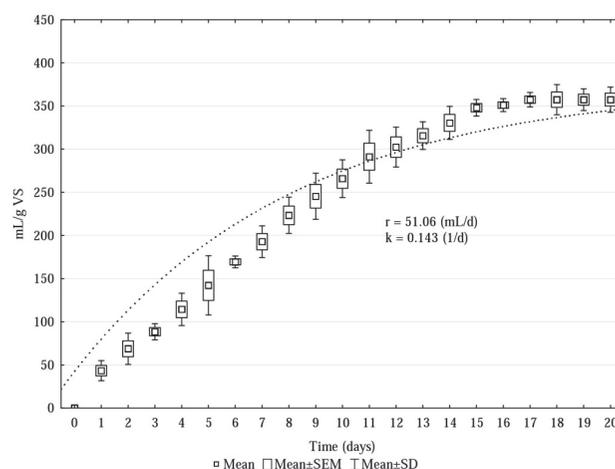
Fig. 3. Cumulative biogas yield of anaerobic digestion of *Bacillariophyceae* in the 20-day test
