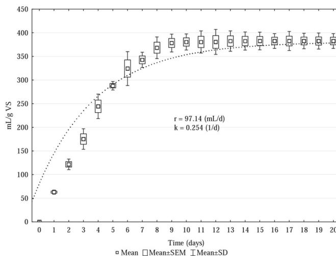
**Fig. 1.** Cumulative biogas yield of anaerobic digestion of *Chlorophyta* in the 20-day test
