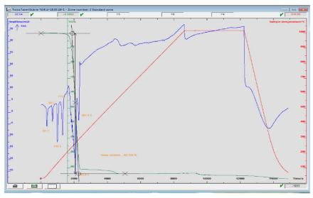
Fig. 10. TGA analysis of ammonium nitrate with 0.01% polyethylene glycol additive
