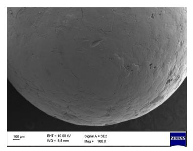
Fig. 8. SEM image of ammonium nitrate with 0.01% carboxymethyl cellulose additive
