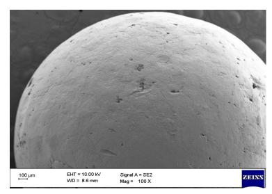
Fig. 9. SEM image of ammonium nitrate with 0.01% polyethylene glycol and 0.01% carboxymethyl cellulose additive
