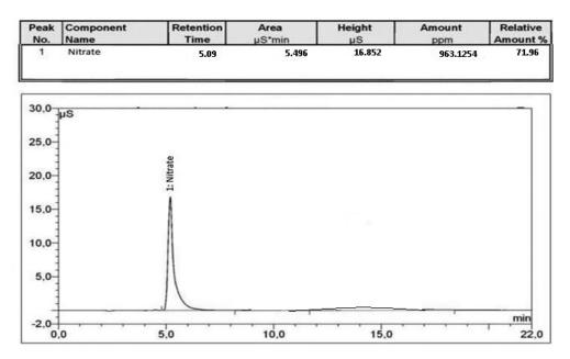
Fig. 4. Ion chromatography of ammonium nitrate with 0.01% carboxymethyl cellulose
