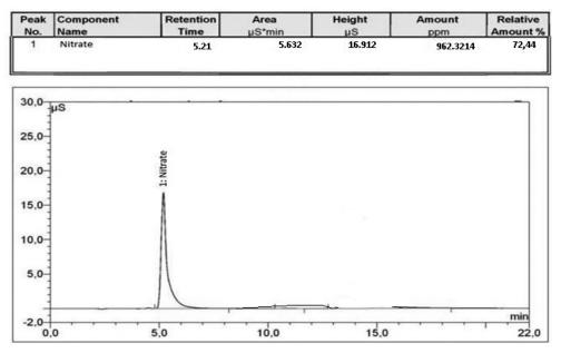
Fig. 2. Anion analysis in ion chromatography of pure ammonium nitrate
