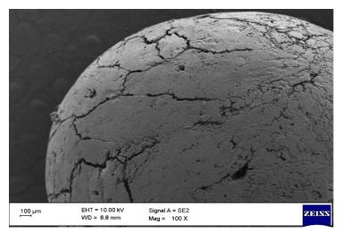
Fig. 6. SEM image of pure ammonium nitrate produced by two-stage evaporation
