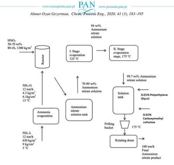
Fig. 1. Ammonium nitrate production with two-stage evaporation method (Gezerman, 2020)
