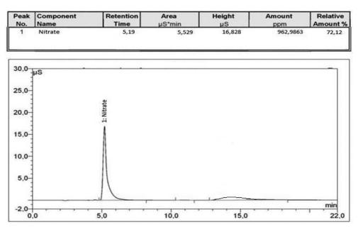
Fig. 3. Ion chromatography of ammonium nitrate with 0.01% polyethylene glycol additive
