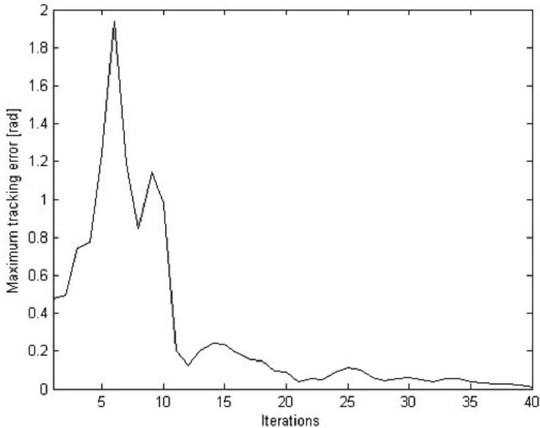
Figure 1: The transient growth error problem of ILC [14]
