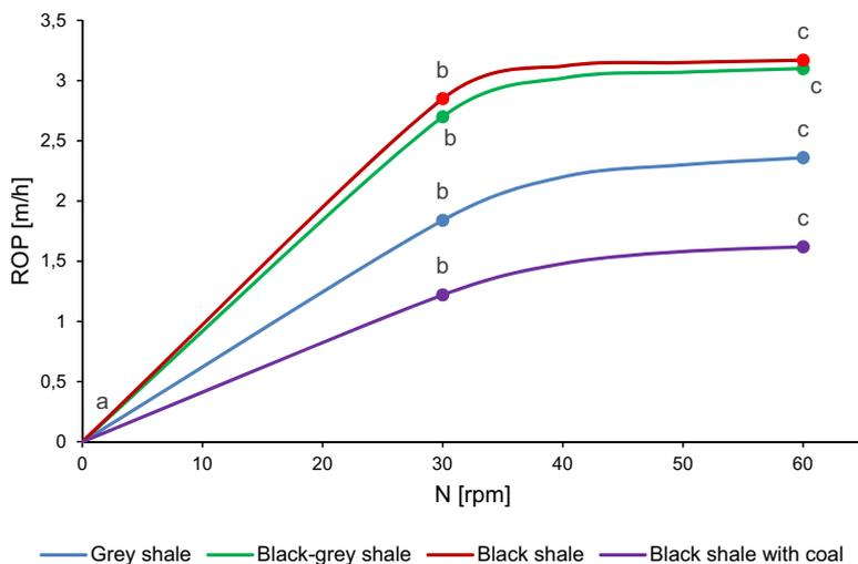
Fig. 11. Result of drillability test.  $WOB - 0.5$  t,  $N \in 30+60$  rpm
