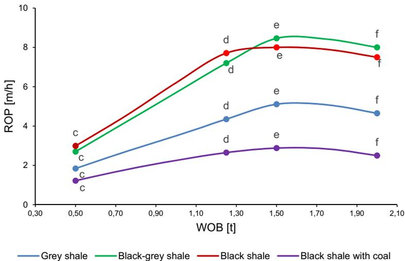
Fig. 9. Result of drillability test. *N* – 30 rpm, *WOB* ∈ 0.5÷2.0 t
