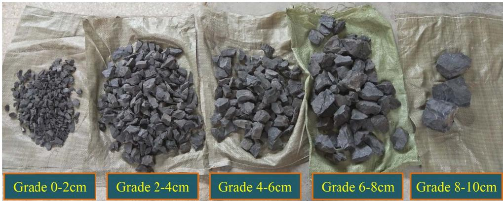
Fig. 1. Distribution of crushed sandstone grades
