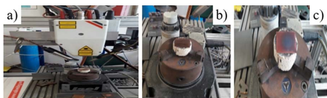
Fig. 1. Laser-treatment processing: a) a view of experimental stand equipped with a 2.0 kW continuous wave high power direct laser, b) ceramic table with deposited sample before the process, c) sample after the process (example)
