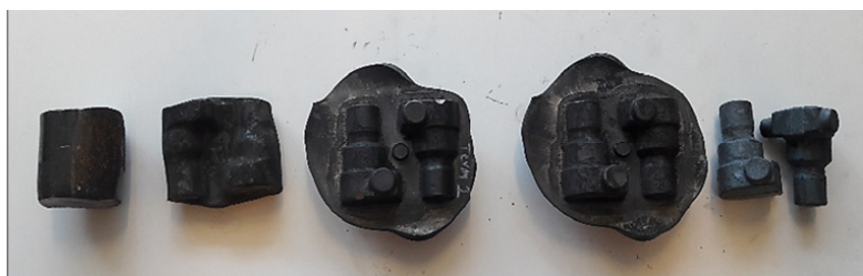
Fig. 5. Appearance of forgings after each forging operation
