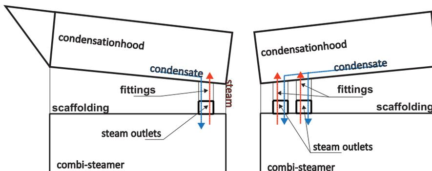
Figure 4: Scheme of the condensation hood position relative to the combi-steamer with scaffolding; outlet channel not included: left-hand side – side view, right-hand side – rear view.
