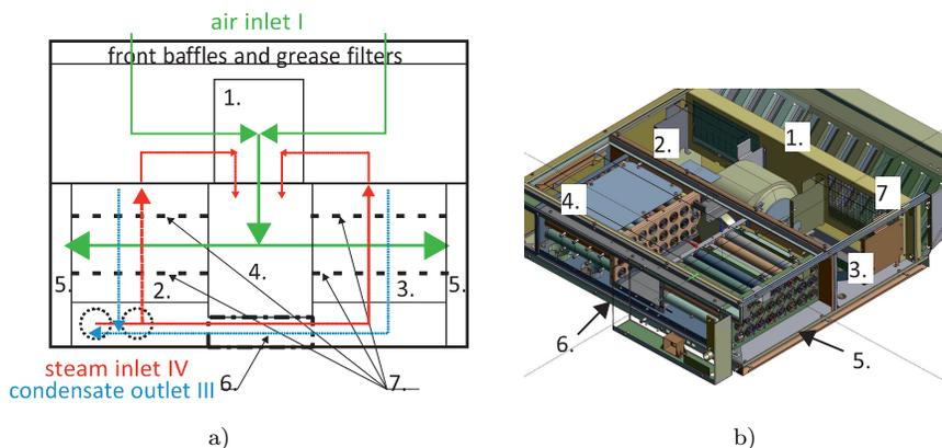
Figure 1: Condensation hood: a) top schematic view, b) isometric view; 1 – fan, 2, 3 – bundles of pipes, 4 – air distribution chamber, 5 – peripheral air chambers, 6 – steam channel; 7 – steam baffles.
