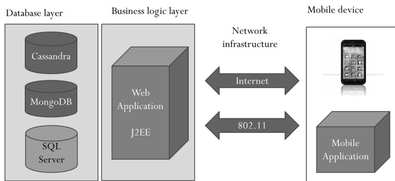
Fig 1. Three-layer architecture and access to databases.
