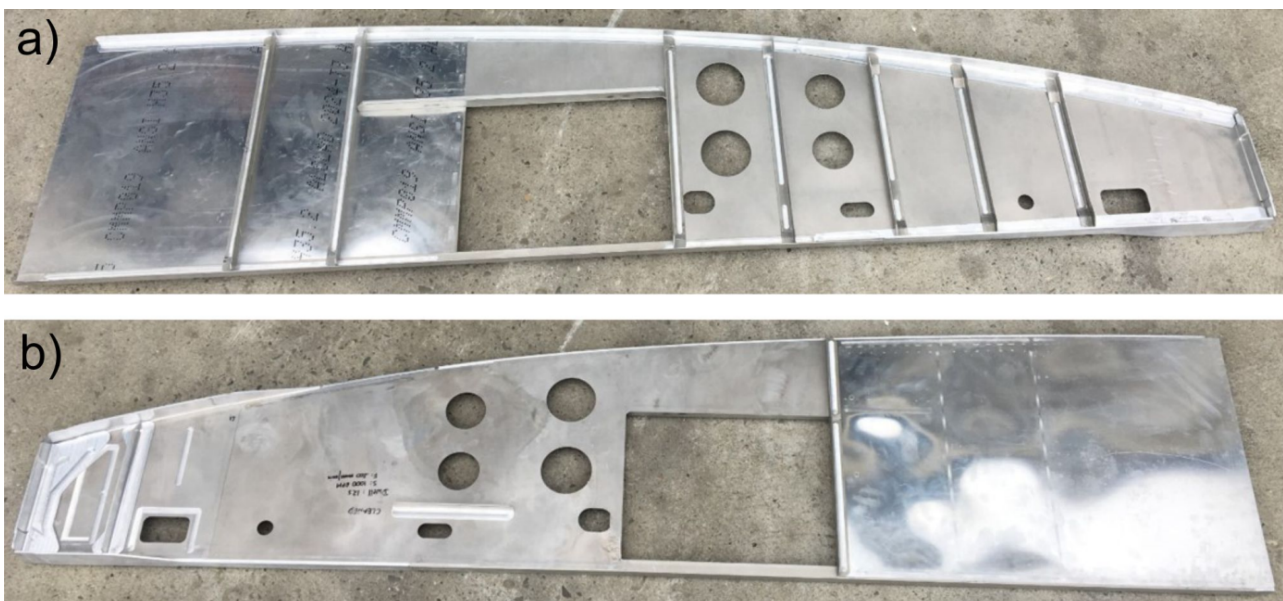
Fig. 15. View of the welded elements of the M28 aircraft landing gear beam (demonstrator), a) front side, b) back side
