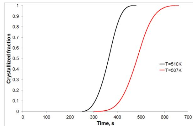
Fig. 6. The crystallized volumetric fraction as a time function for various isothermal annealing temperatures of Mg<sub>72</sub>Zn<sub>24</sub>Ca<sub>4</sub> alloy
