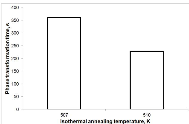
Fig. 8. Duration of the heat effect depending on the isothermal annealing temperature
