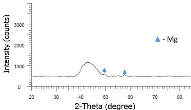
Fig. 1. Results of X-ray diffraction for Mg<sub>72</sub>Zn<sub>24</sub>Ca<sub>4</sub> ribbon sample
