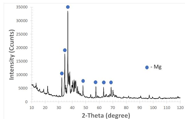
Fig. 2. Results of X-ray diffraction for Mg<sub>72</sub>Zn<sub>24</sub>Ca<sub>4</sub> ribbon after isothermal annealing at 507 K
