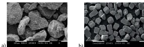
Fig. 1. SEM images of: (a) reinforcing phase  $\text{Al}_2\text{O}_3$  particles with average size of 10-30  $\mu\text{m}$ , (b) NaCl particles. in the range of 500–1000  $\mu\text{m}$
