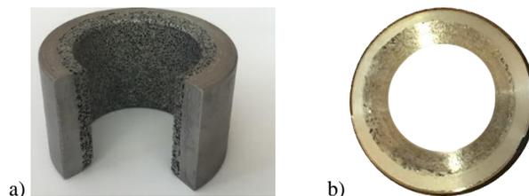
Fig. 3. Materials for tests: (a) element with outer pores free region and thin inner high porosity open cell region; (b) element of outer pores free region and inner hybrid region which consists of babbitt infiltrated open cell skeleton
