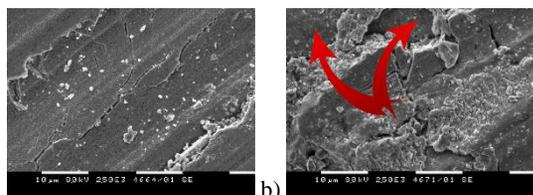
Fig. 5. SEM images of samples after conducted wear tests: (a) pure babbitt, (b) infiltrated with babbitt skeleton
