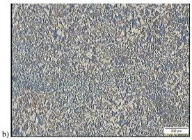
Fig. 4. The microstructure of cast steel with a micro-additive of 0.1% V: a) in the initial state, b) after normalization; marker 200 µm
