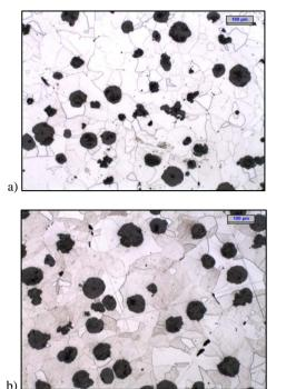
Fig. 5. The microstructure of the strength ingot adhered to the surface of the slag ladle: a) slag ladle with a capacity of 3.6 m<sup>3</sup>, b) slag ladle with a capacity of 11 m<sup>3</sup>
