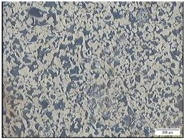
Fig. 3. The microstructure of cast steel without V in the initial state a) and after normalization, b) marker 200 µm
