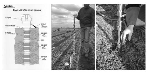
Fig. 5. Scheme of Sentek's EnviroSCAN with sensors and EasyAG (right)
