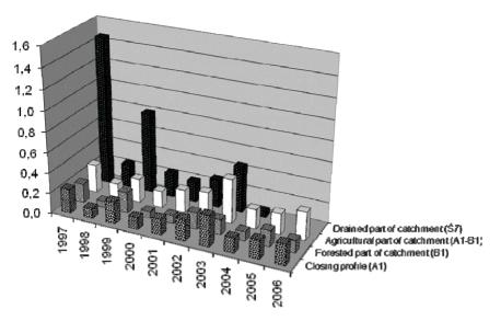
Fig. 3. Mean annual runoff coefficient for individual sections of the Cerhovice stream catchment (1997–2006)
