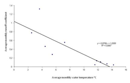
Fig. 7. Runoff coefficient dependence on water temperatures – the Cerhovice stream; hydrological year 2003
