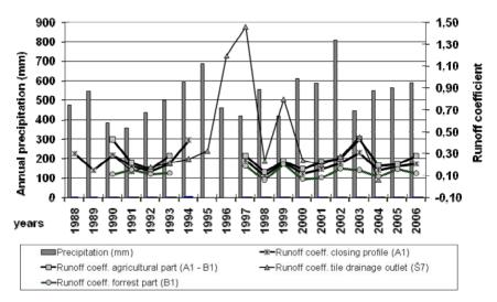
Fig. 2. Runoff coefficient and precipitation at the Cerhovice stream (1988-2006)
