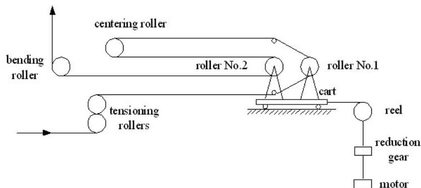
Fig. 1. Kinematic diagram of the loop device
