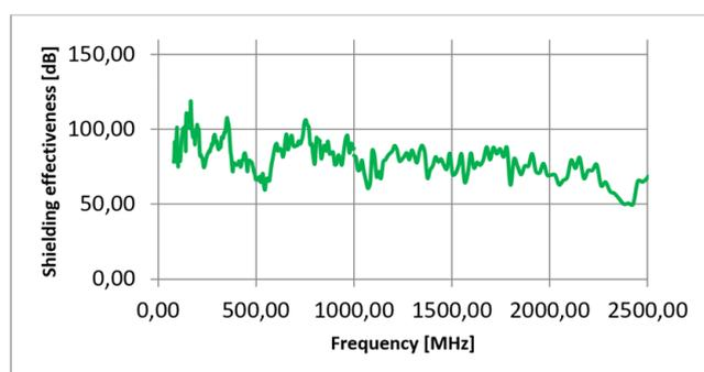
Fig. 7. Resulting  $A_s$  of the shielding enclosure.
