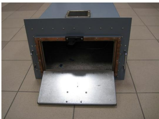
Fig. 6. External view of the front panel of the shielding enclosure.
