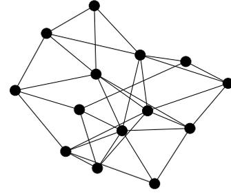
Fig. 5. (net1) Network topology with 14 switch nodes and 64 directed links
