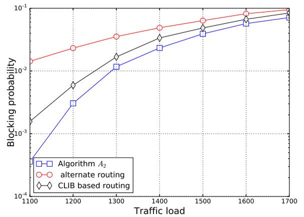
Fig. 19. Comparison of blocking probabilities obtained from RSA algorithm  $A_2$ , alternate routing, and CLIB based RSA in net3
