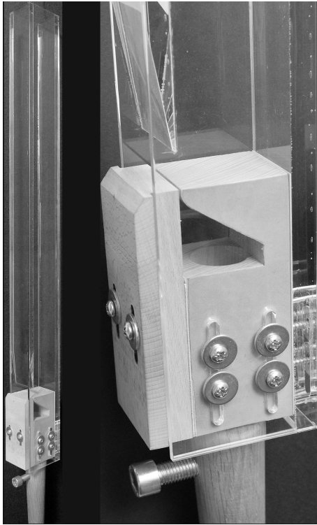
Fig. 4. The experimental flue organ pipe and detail of its mouth region.
