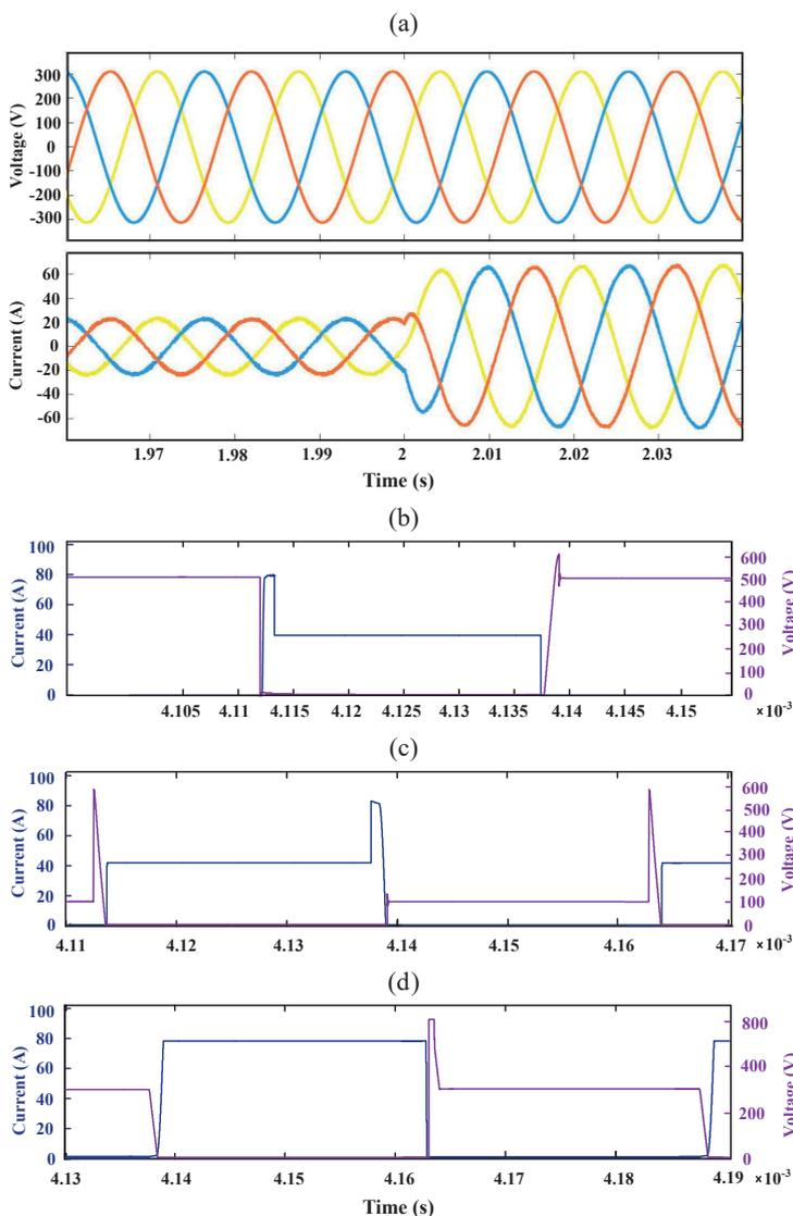
Fig. 7. Simulated results, (a) input voltage and current, (b) switch current and voltage waveforms, (c) switch diode current and voltage, and (d) rectifier diode current and voltage waveforms
