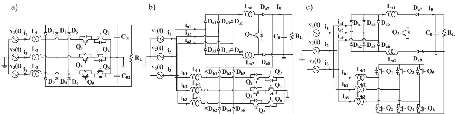
Fig. 1. Prior art high power rectifier topologies, (a) an active three level vienna boost converter system, (b) a hybrid system based on a single switch boost and vienna rectifier units, and (c) a hybrid rectifier system employing a single switch boost and FB boost converter units
