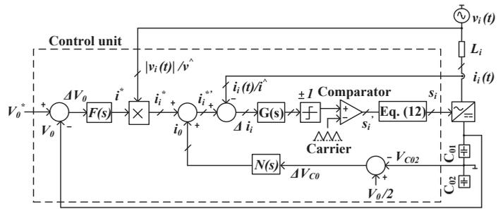
Fig. 6. Control scheme of the proposed soft switched PWM AC/DC converter,  $F(s)$ : controller of output voltage  $V_0$ ;  $N(s)$ : balancing controller of output DC link capacitor voltages  $V_{C01}$ ,  $V_{C02}$ ;  $G(s)$ : current controller of the phase currents  $i_i(t)$ ,  $i = 1, 2, 3$ ;  $s_i$ : switching signals generated according to (12) and (13); the three phase signals are shown by cross lines, for the sake of clarity
