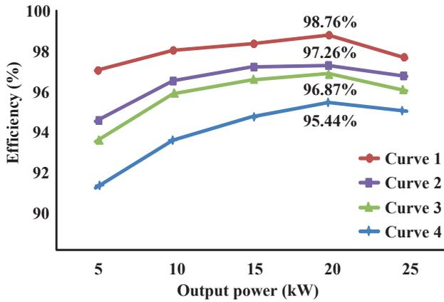
Fig. 13. Efficiency curves of high power converters, Curve 1: Proposed soft switched PWM AC/DC converter, Curve 2: Hybrid system based on FB boost converter, Curve 3: Hybrid vienna based rectifier system, Curve 4: Three level vienna rectifier system
