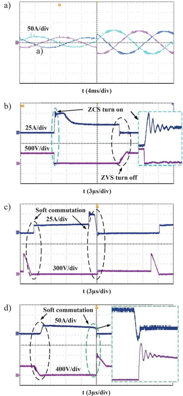
Fig. 15. Experimental results, (a) grid injected current dynamic response, (b) semiconductor switch current and voltage, (c) semiconductor switch diode current and voltage, and (d) rectifier diode current and voltage waveforms
