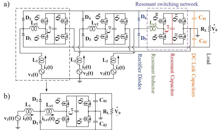
Fig. 2. (a) Proposed soft switched PWM AC/DC converter, (b) Decoupled single phase configuration of the proposed soft switched PWM AC/DC converter
