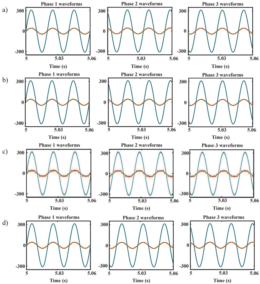
Fig. 8. Grid injected current and voltage waveforms, (a) three level vienna boost rectifier, (b) proposed soft switched PWM AC/DC converter, (c) hybrid rectifier system based on three level vienna rectifier, and (d) hybrid rectifier system based on FB boost converter
