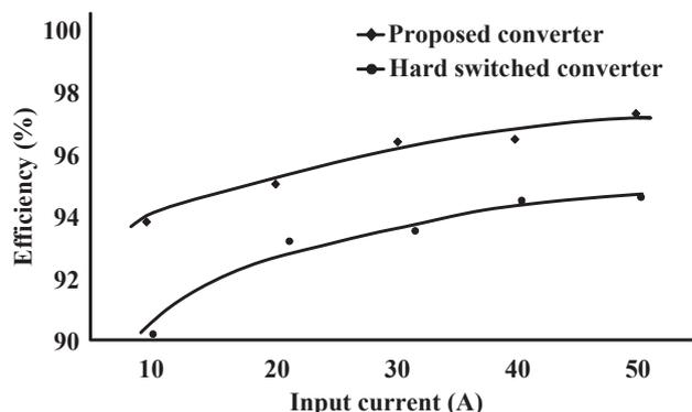
Fig. 19. Efficiency comparison of the proposed soft switched and hard switched PWM AC/DC converters
