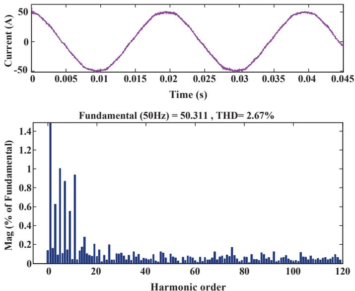
Fig. 18.  $THD_I$  of the proposed soft switched PWM AC/DC converter
