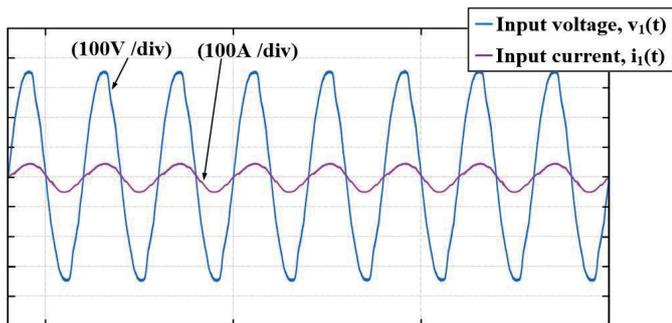
Fig. 16. Grid voltage and current waveforms of the proposed soft switched PWM AC/DC converter showing PFC operation
