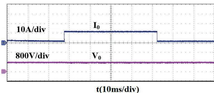
Fig. 17. Output characteristic of the proposed soft switched PWM AC/DC converter
