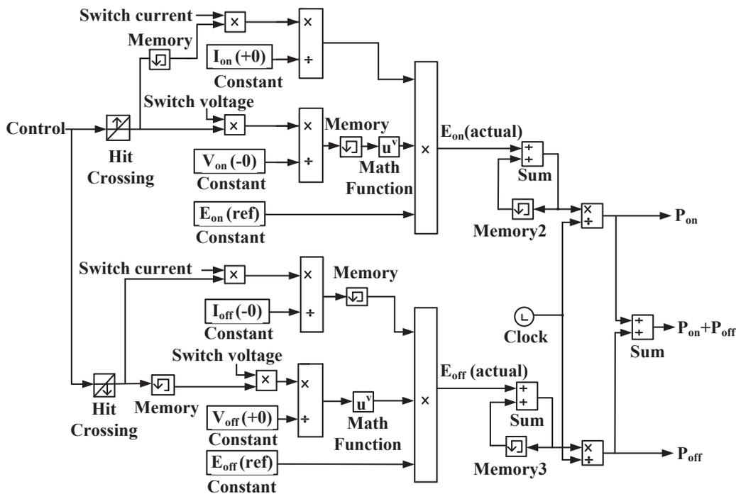
Fig. 11. Simulink system block for  $E_{on}$ ,  $E_{off}$  and average power loss calculation
