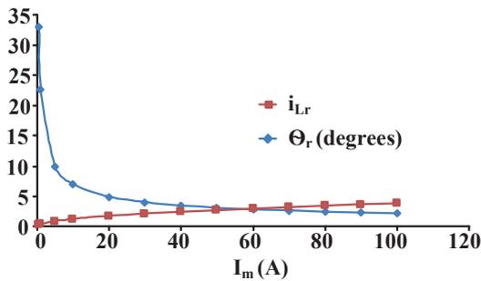
Fig. 5. Curve representing effectiveness of resonant inductor current near zero crossing
