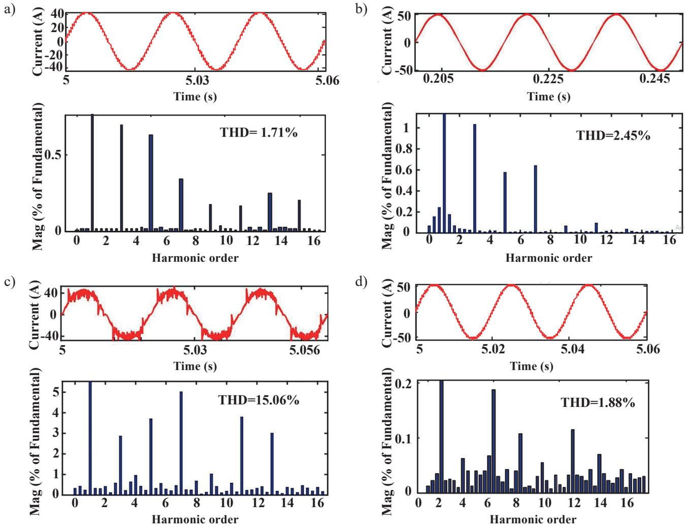
Fig. 10. Input current harmonic analysis, (a) three level vienna boost rectifier, (b) proposed soft switched PWM AC/DC converter; (c) hybrid vienna based rectifier system, and (d) hybrid rectifier system based on FB boost converter
