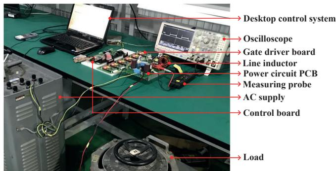
Fig. 14. Experimental setup diagram of the proposed soft switched PWM AC/DC converter
