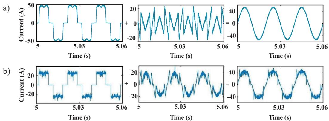
Fig. 9. Composition of the desired sinusoidal waveform from input current waveforms of compounding units, (a) hybrid rectifier system based on FB boost converter, and (b) hybrid vienna based rectifier system
