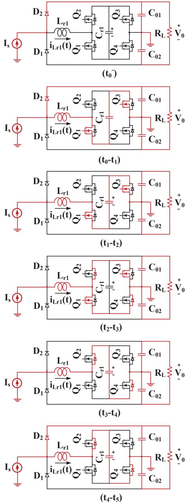
Fig. 4. Equivalent circuits corresponding to various stages of the proposed converter scheme during positive half cycle of the input voltage
