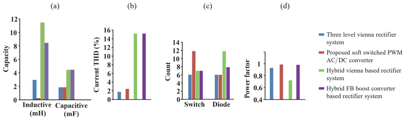
Fig. 12. Graphical illustrations, (a) energy storage passive components capacities, (b) input current THDs, (c) semiconductor device and rectifier counts; and (d) power factor corrections of the high power converter topologies
