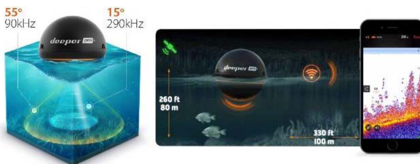
Fig. 6. Sonic depth sounder used for field measurements; source: own elaboration
